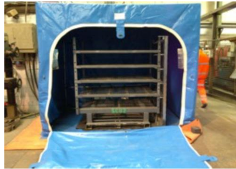
Fresh Solidia Concrete in contact with CO 2 (24h)
